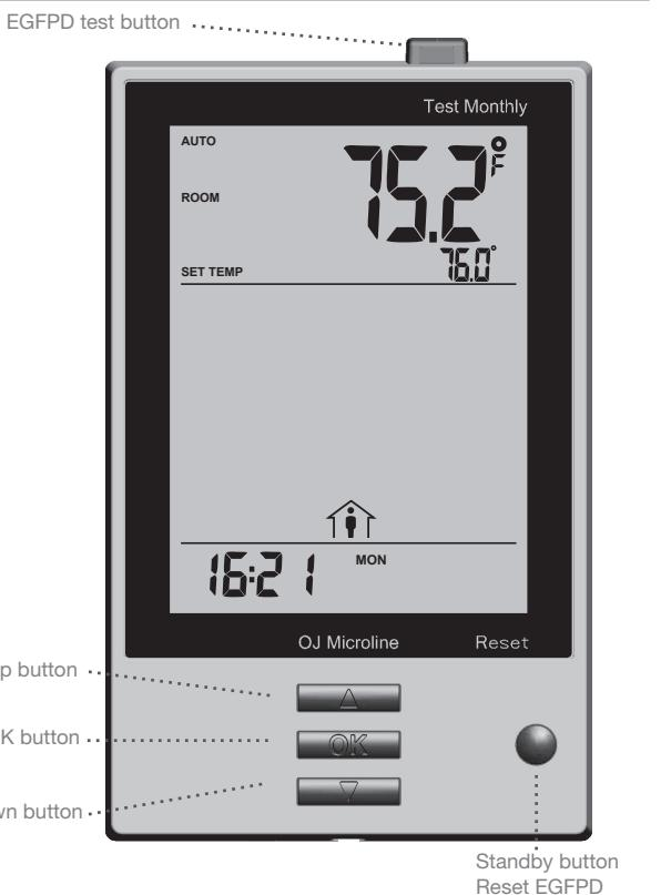
Adjust the setpoint until the heating symbol (SSS) appears. Use the **Up** button to increase the heating demand and then press the **OK** button. Wait 10 seconds to allow the thermostat to adjust to the new setpoint. Then press the **TEST** button on the top of the thermostat.
