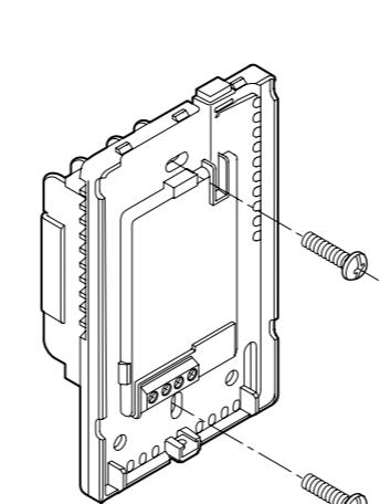
Install the power base into the electrical box.
